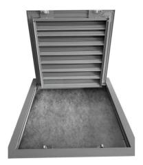
The filter is mounted between the hinged grille and the wire mesh. For filter replacement open the grille by pressing on mini-latches system.
