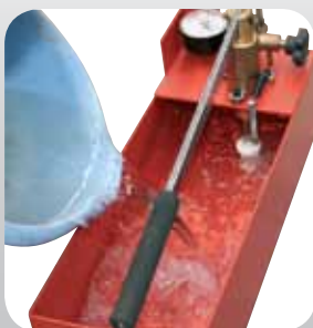
1-Fill up the tank
