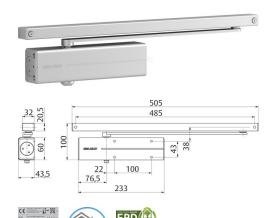
Rack and pinion door closer with guide rail
