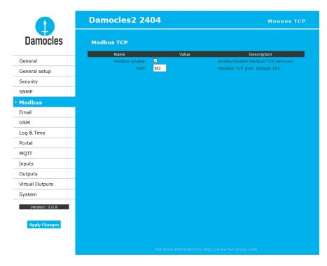
Note: The Modbus/TCP protocol is not secured in any way. We do not recommend using it outside of an isolated network. For basic security, it can be combined with the IP address filter.
