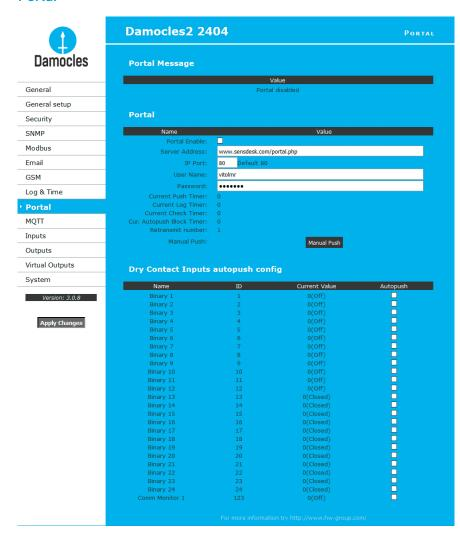
Configures the communication with the portal using the HWg-Push protocol. Damocles2 is the active side and establishes communication periodically and upon every DI change.
