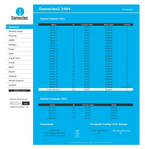
The main page with the overview of DI and DO states automatically reloads at configurable intervals (by default every 10 seconds, can be changed easily).
