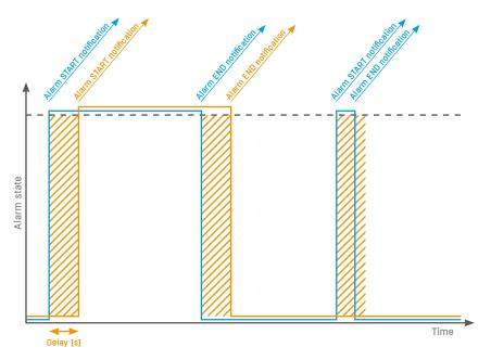
Alarm status notification based on a Delay value:
