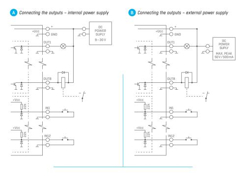
Connecting Damocles2 1208 units (OC outputs) to Poseidon2 (DI inputs)
