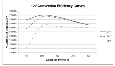
1. Solar Module MPP Voltage(17V, 34V, 68V) / Nominal System Voltage(12V)
