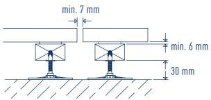
The butt joint should never be installed on the substructure and with a distance of at least 7 mm!
