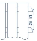
The joint distance for plank widths 90 - 120 mm should be at least 7 mm or 6% of the plank width!
