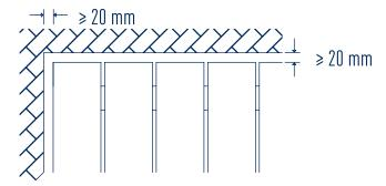
When connecting the terrace to the adjacent building, a distance of  $\ge 20$  mm must be observed so that the joints cannot close either through dirt or changes to the planks. The unhindered drainage on and beneath the terrace must be permanently guaranteed.
