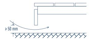
If the side of the terrace is closed with a cover board, a ventilation opening of  $\geq$  50 mm (continuous) must be maintained for ventilation of the terrace construction. The cover board should not touch the ground.
