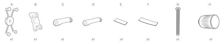
Select proper strap (C or D) and rubber strip (E or F) to fit the following rail diameters:
