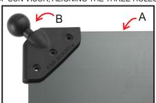
3. ATTACH (B) BALL BASE TO (A) SUN VISOR SCREEN USING (C) SCREWS AND (D) NUTS.
