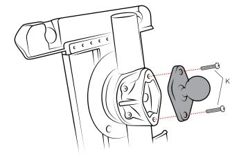
8 Attach keyboard to (C) RAM® Power Plate™ III. When positioning (G) tube, take into account the amount of space needed to rotate your tablet between portrait and landscape mode.
