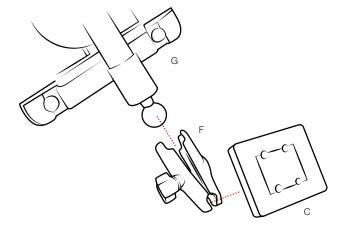
6 Determine proper height adjustment by sliding (G) tube up and down as needed. When set to the correct position, evenly tighten the (J) screws behind (A) RAM® Roto-View™.
