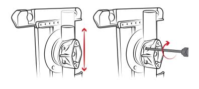
7 Attach your RAM® ball base to the holes behind (B) tube adapter using (K) screws.
