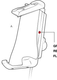
GREEN: Phone is charging RED: Holder detects power FLASHING RED: Error
