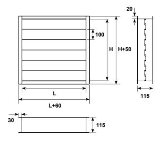
Dimensions  $\mathbf{L}$  x  $\mathbf{H}$  are duct dimensions. Volume damper internal dimensions:  $\mathbf{L}$  x ( $\mathbf{H}$ +10)
