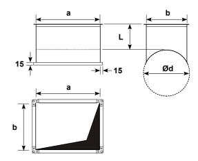
Dimensions **a** x **b** are measured without flanges. **L** standard - 100 mm
