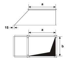
Dimensions **a** x **b** are measured without flanges. **L** standard - 100 mm
