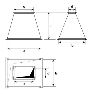
Dimensions **a** x **b** / **c** x **d** are measured without flanges.
