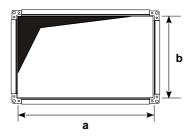
Dimensions **a** x **b** are measured without flanges.
