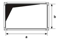
Dimensions **a** x **b** are measured without flanges.
