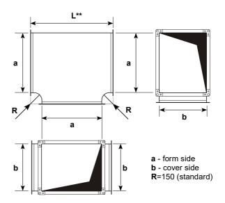
Dimensions  ${\bf a} \times {\bf b}$  are measured without flanges.
