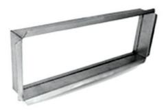
For mounting the CC frame of a grille with sizes LxH (mm), a opening hole with (L+5)x(H+5) mm is needed.
