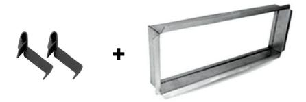
For mounting the CC frame of a grille with sizes LxH (mm), a opening hole with (L+5)x(H+5) mm is needed.
