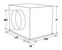
Ød - flexible duct connection diameter (mm)
