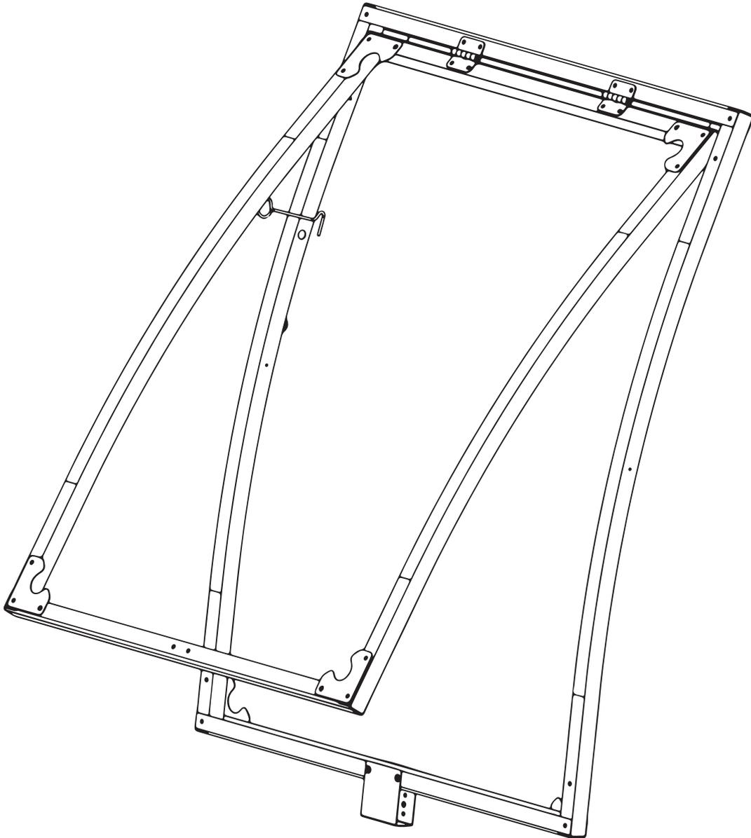
The vent for the greenhouse "ComfortProm" is designed to the Greenhouse ventilation and is installed in the roof of the greenhouse with self-tapping screws with a press washer and a rubber seal. Covered with cellular polycarbonate.
