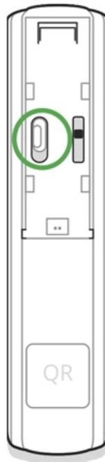
For detection and pairing to occur, the detector should be located within the coverage area of the wireless network of the hub (at a single protected object). The connection request is transmitted for a short time: at the moment of switching on the device.
