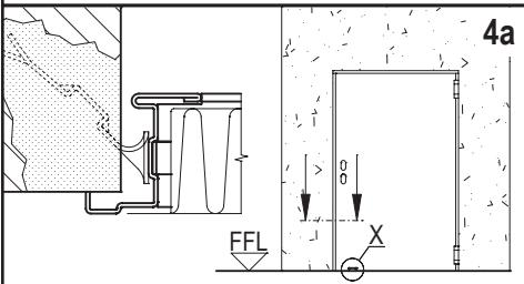
Insert a 10mm spacer under the door leaf with FM  $L \geq 1000\text{mm}$  (X). Temporarily immobilise the door in the wall opening, respecting the plumb-line, the FFL level and the parallelism to the wall. Fix the anchors with quick set cement.
