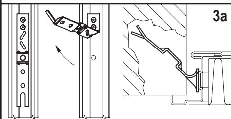
Bend up the frame anchors and mark on the wall their positions respecting the FFL level. Create the holes in the wall for the anchors.
