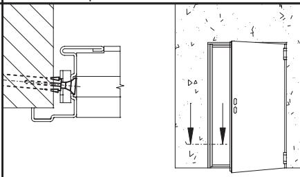
Open the door-leaf and fix the frame at presetted holes with expansion screws type Würth art. 0910436112 (expansion screws not supplied), starting with the jamb from hinges side. Close again the door-leaf.
