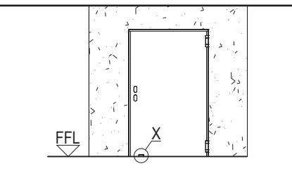
Insert a 10mm spacer under the door leaf with FM  $L \geq 1000\text{mm}$  (X). Temporarily immobilise the door in the wall opening, respecting the plumb-line, the FFL level and the parallelism to the wall.
