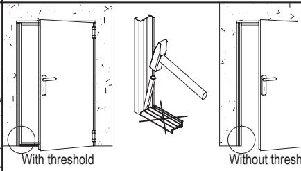
**Warning: the threshold does not be removed in case of door with environmental characteristics.**
