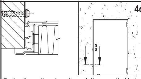
Fasten the wall anchors through the preset holes, using plastic expansion screws Hilti, HRD-UGS Ø10x100mm and the doorframe in hinges zone, using the Würth art. nr. 0910436112 steel anchor bolts. Expansion screws and anchor bolts are not supplied.
