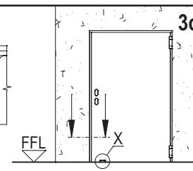
Insert a 10mm spacer under the door leaf with FM  $L \geq 1000\text{mm}$  (X). Bend the wall anchors appropriately, temporarily immobilise the door in the wall opening, respecting the plumb-line, the FFL level and the parallelism to the wall.
