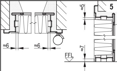
Fill up the space between doorframe and wall with mortar, without bending the frame, cover the frame with plaster and check the leeway.
