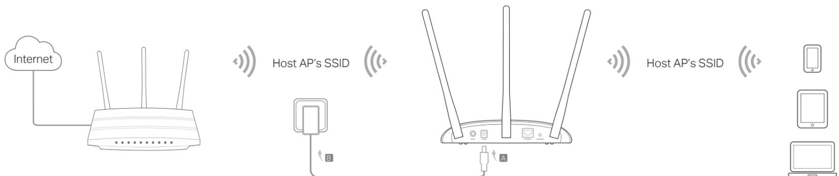
1. Connect the access point according to Step A and B in the diagram.
