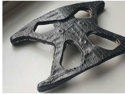
(b) Steering wheel moulded without a mould using two layers of a thicker fiber
