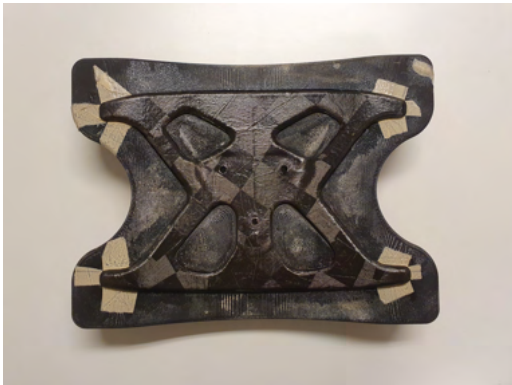
(c) Finished steering wheel body in the mould after curing
