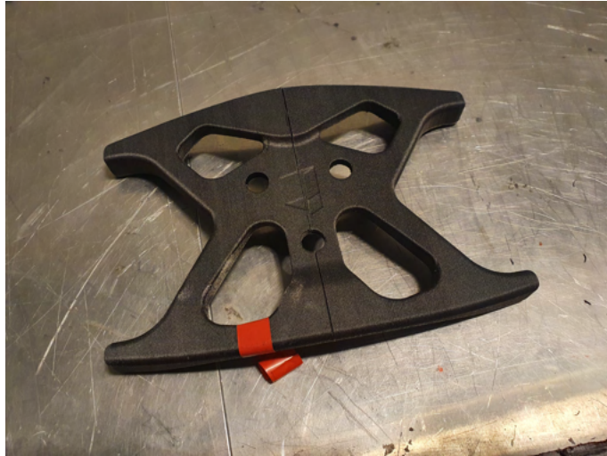
Figure 8: Steering wheel core with 0.5mm offset glued together
