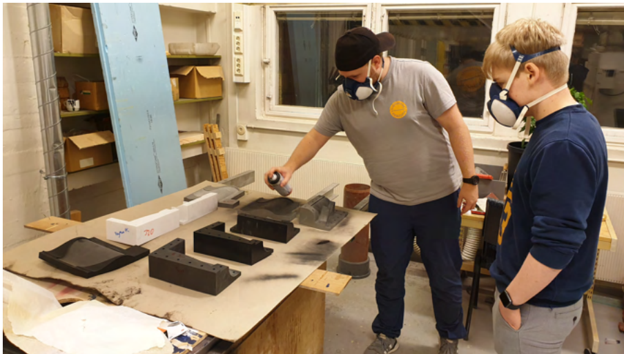
Figure 3: Spraying process using the Hagemans Spraymax 2K Epoxyprimer Filler
