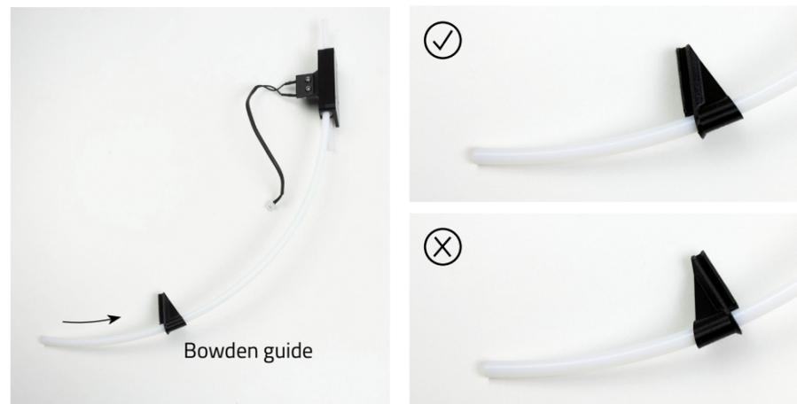
4.2 Screw the new printed part "Bowden entry" provided with the kit on the lateral covers with the two screws used in the step (2.9) as shown in the picture, with the orientation indicated (notch inwards).
