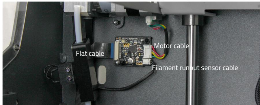
4.12 When connecting the flat cable, remember to open the tab of the driver as indicated in the following picture.
