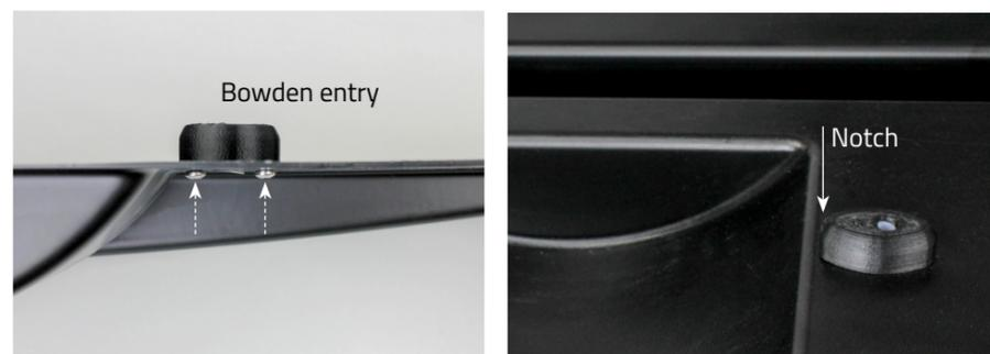
4.3 Insert the new teflon tube with the filament sensor into the "Bowden entry". Press until you feel that you have reached the end.
