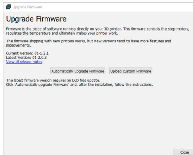
3.1.5 Wait until the firmware is installed. The process may take a few minutes to complete.
