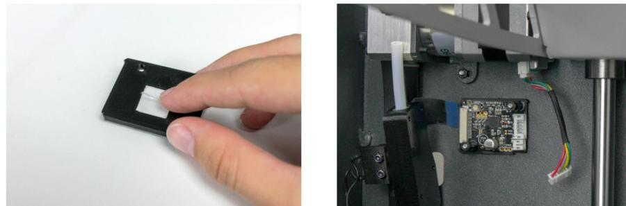
4.11 Connect the flat cable, and then connect the motor cable and the filament runout sensor cable as indicated the picture.
