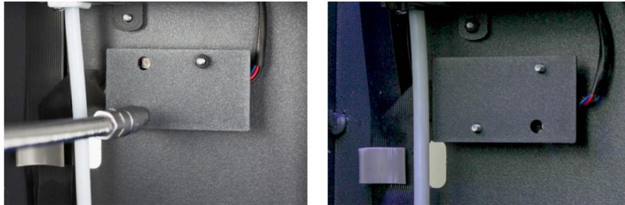
2.2 Disconnect the flat cable that goes to the driver, opening the tab that fixes it. Also disconnect the motor cable connector.
