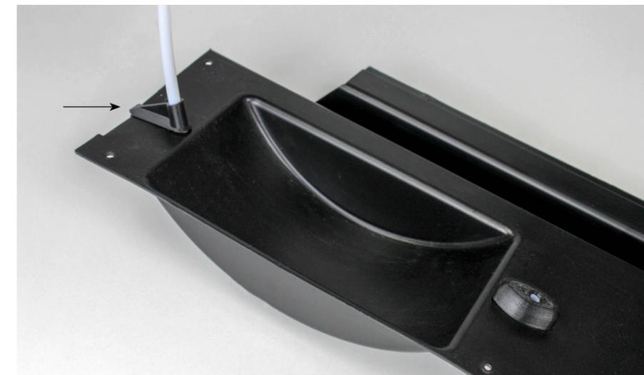
4.5 Before carrying out this step, make sure that the brackets are placed with the flat side facing up. Place the side covers. To do this, place the cover as shown in the image. Then, push on the side indicated in the picture.
