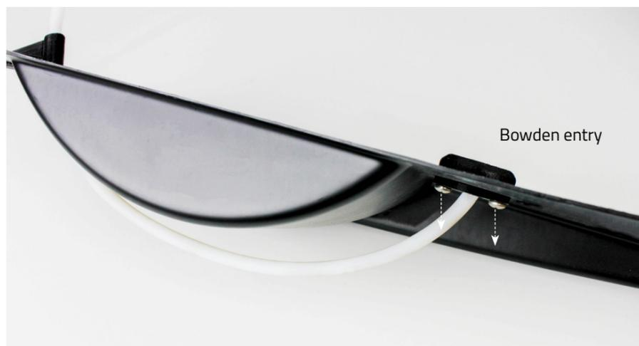
2.10 Remove and keep the printed part "Bowden guide" from the lower teflon tube. Don't keep the lower bowden tube, as it won't be used again.
