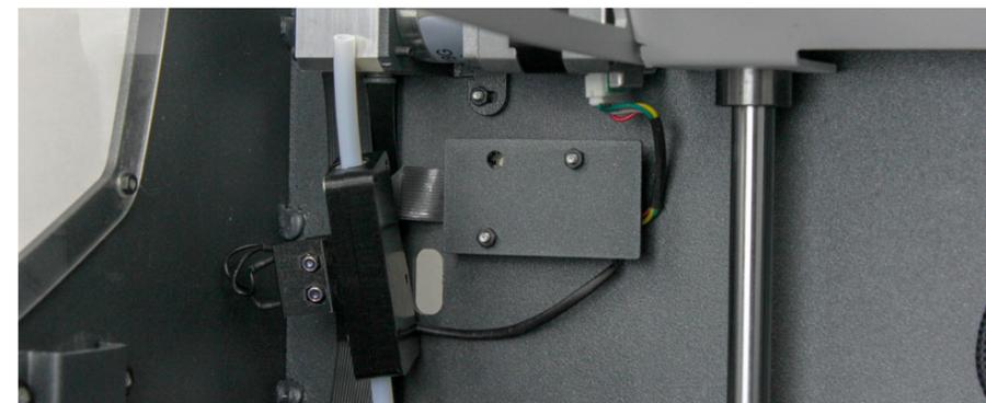
4.14 Insert the lower teflon tubes, making sure they are properly placed. Finally, place the new black clips provided with the kit both above and below the extruder.
