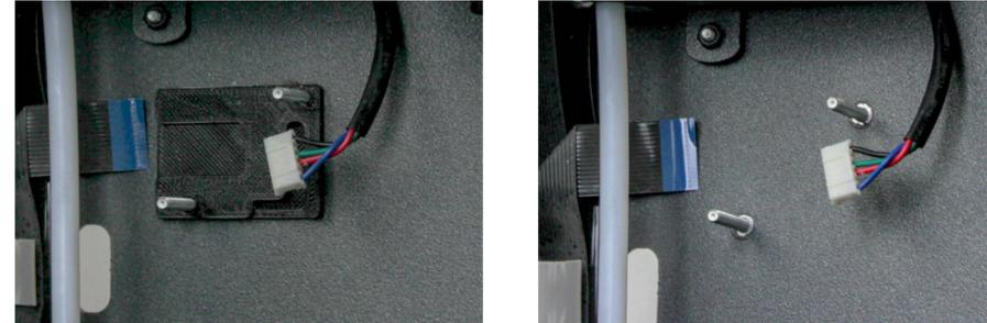
2.4 Remove the lower teflon tube from both sides. To do this, hold down the coupling with your fingers and pull out the tube.
