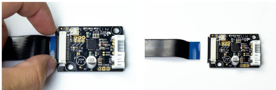
2.3 Remove the driver and the driver spacer (black piece). Do not keep these parts, as they will not be used again.
