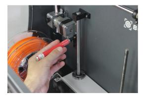
**4.** Clean grease and dust from the Z-axis motor spindle with paper or a cloth. Turn the spindle manually to access its rear.
