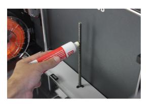
**6.** Turn on the Sigma and from the LCD screen, go to *Utilities --> Maintenance--> Move printing surface.* Raise and lower the platform twice to evenly distribute the oil and grease. Finally, remove the remnant grease.
