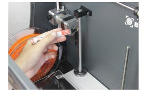
**3.** Apply the lubricating oil pencil along the Z shaft bars, making sure that it does not drip.
