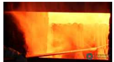
Figure 8. Sinter the ceramic shell and burnout
