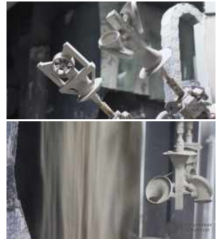
Figure 7. Make the ceramic shell
