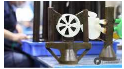
Figure 6. Adhere the PolyCast™ pattern to the wax tree
