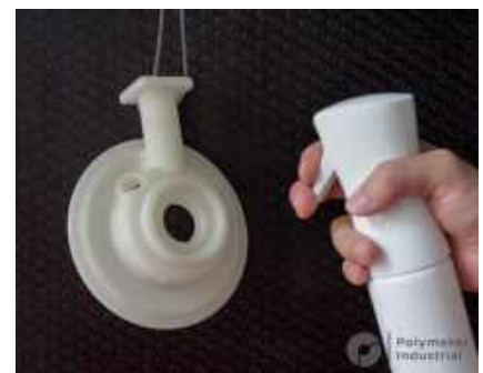
Figure 5. Spray isopropyl alcohol on the PolyCast™ pattern
