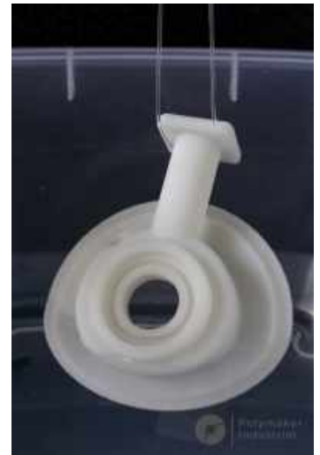
Figure 4. Dip the PolyCast™ pattern into isopropyl alcohol
