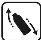
The composition of the resin can contain suspended particles, over time these can end up precipitating at the bottom of the container, so it is advisable to shake the container before use so that the product mixes again and is completely homogeneous.
