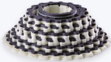
Bicycle cassette model before support material dissolution
