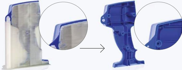
An end-use power tool handle before and after soluble support removal
