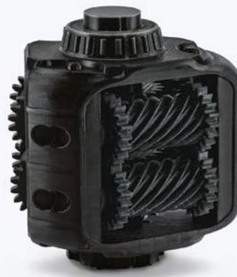
Torsen differential mechanism
