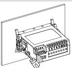
Insert the unit into a panel, fasten the bracket by pushing with tools with a flathead screwdriver.
