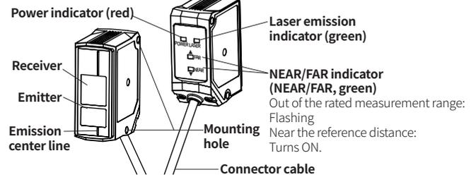
• Emission center line and the object should be aligned because the laser is emitted along the line.
