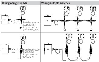
Maximum 30 unit of switches can be connected to a controller (SFC-N322).
