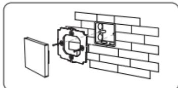
Fix the controller base on the bottom
