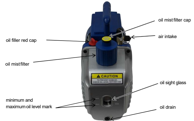
Photo 2: Rotary oil vacuum pump - front view.
