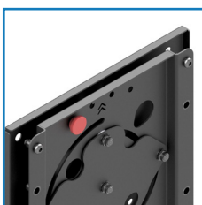
Securing the screen against falling with screws
