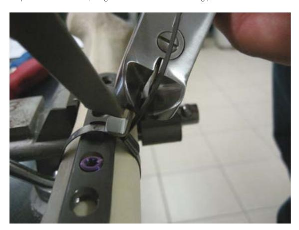
11. Fold the cut end on the band with the bending tool.
