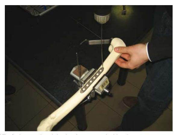
2. Make the pre-drilling for the screw through the sleeve's mono- or polyaxial section.
