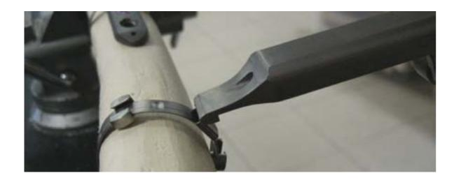
4. Install the spacer and cut the top edge of the band with the cutting pliers.
