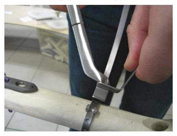
5. Fold the end of the band with the bending tool.
