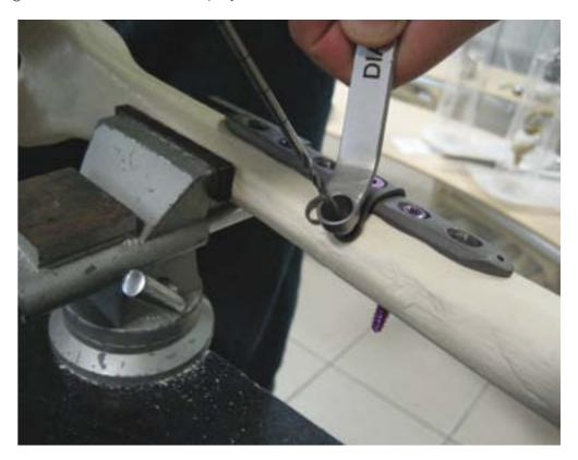
4. Measure the length of the necessary polyaxial screw.
