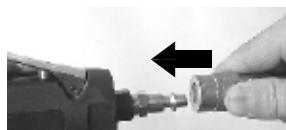
6. Remove the air inlet cap and connect air hose to the device.
