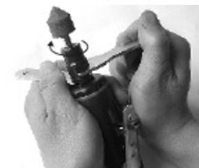
5. Tighten the tip in the device: grip the spindle with a spanner and then use another spanner to grab the flange and twist in a clockwise direction.
