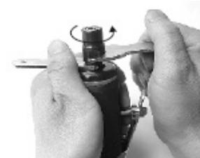
3. Unscrew the flange: grip the spindle with a spanner and then use another spanner to grab the flange and twist in an anticlockwise direction.
